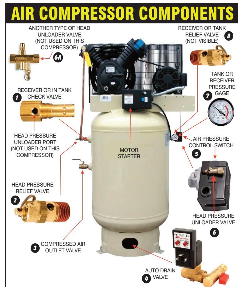
a cylinder, compressing the air in front of the piston head; just the reverse principle of the gasoline engine.
