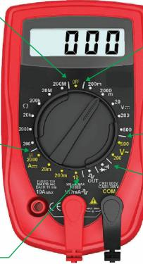
This is the range of settings for measuring VOLTS DC. The symbol for VOLTS DC is using this range since most of the voltage measurements you'll be taking will be in volts AC.
