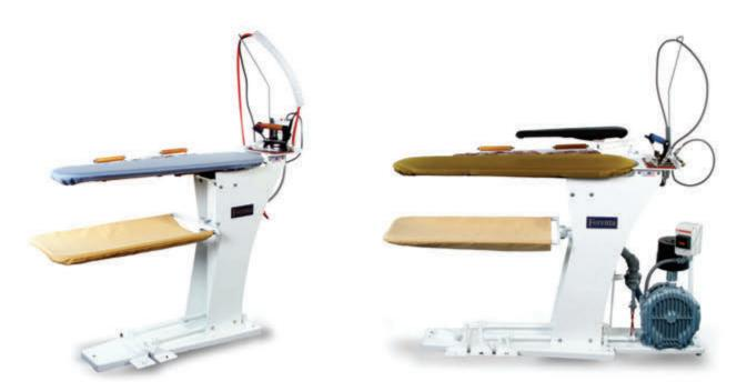
Steam-heated buck design with flat surface
