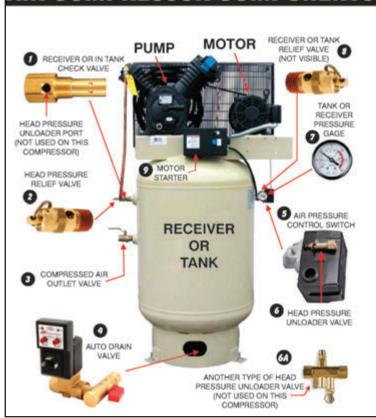
There are some compressors (usually larger types) that, when the desired pressure is reached the motor continues to run. However, the cylinder head is unloaded to the atmosphere using an unloader valve (see item 6a) so there will be no further increase in tank pressure
